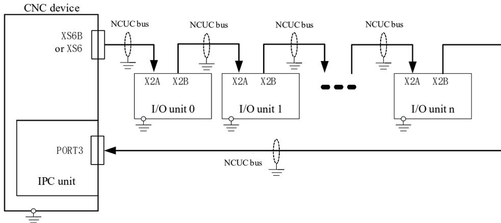
Fig. 2.2 Connection diagram of CNC controller and bus I/O unit
