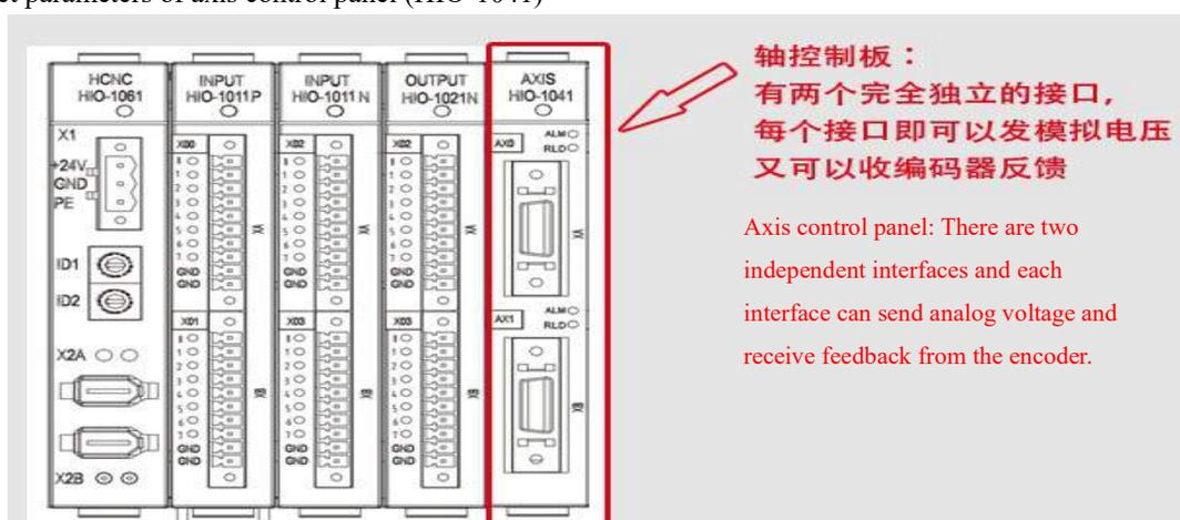
If only HIO-1041 control panel is connected, parameters are configured as below:
