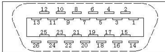
Pin of XS5 spindle motor encoder input interface plug
