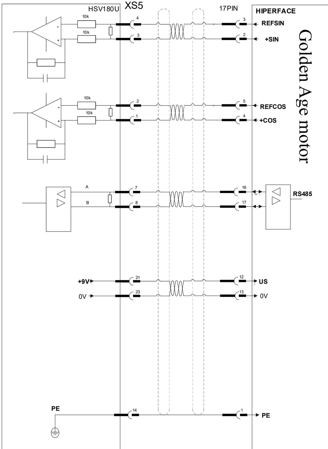
Note: HSV-160UP and HSV-180UD series support this encoder and HSV-160UD series do not support it.
