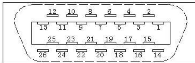
Pin of input interface plug of servomotor encoder
