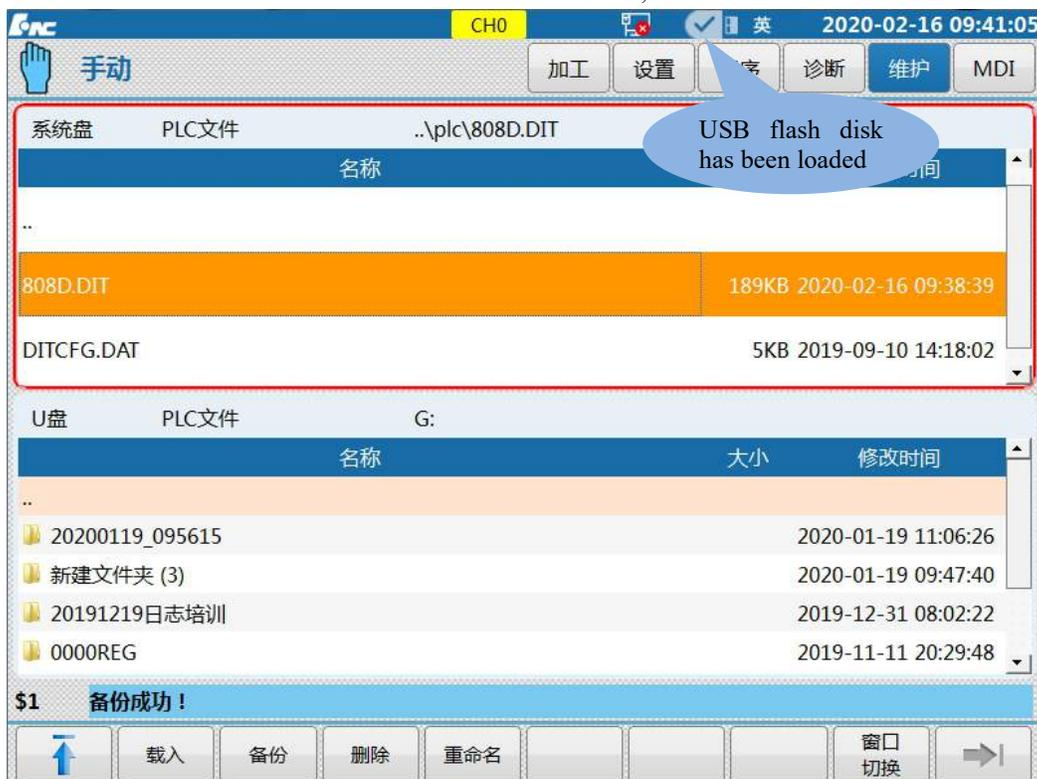
5) Select the file to be loaded by "↑" and "↓" on the NC panel, press "Load" and the system gives a prompt
