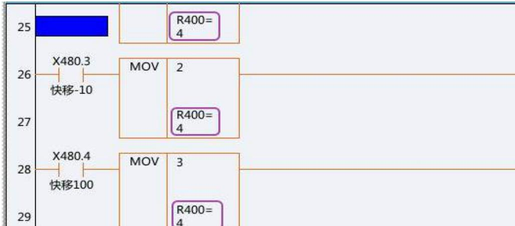
When latched value is displayed, values of registers displayed in the ladder diagram monitoring screen are displayed independently for every module.
