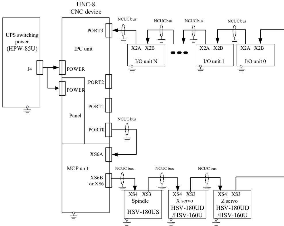
Fig. 2.3 Typical connection between HNC-8 series CNC controller and bus-type I/O unit and bus-type servo drive unit
