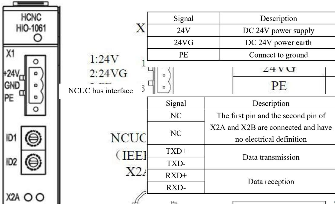
2) Definition of switch value input/output module interface
