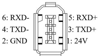
Connection diagram of NCUC bus cable
