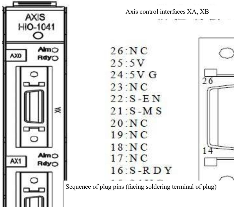
Sequence of plug pins (facing soldering terminal of plug)
