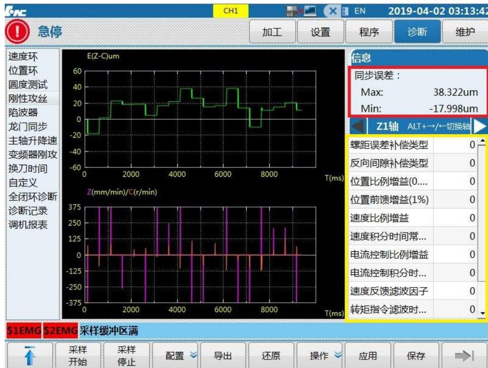
The red box indicates the synchronous error automatically calculated by the system. Z axis or spindle servo gain is adjusted according to the synchronous error so that the value is approximate to the minimum value, then the best condition of interpolation of two axes is reached. The yellow box indicates tapping axis servo gain and acceleration/deceleration adjustment window.
