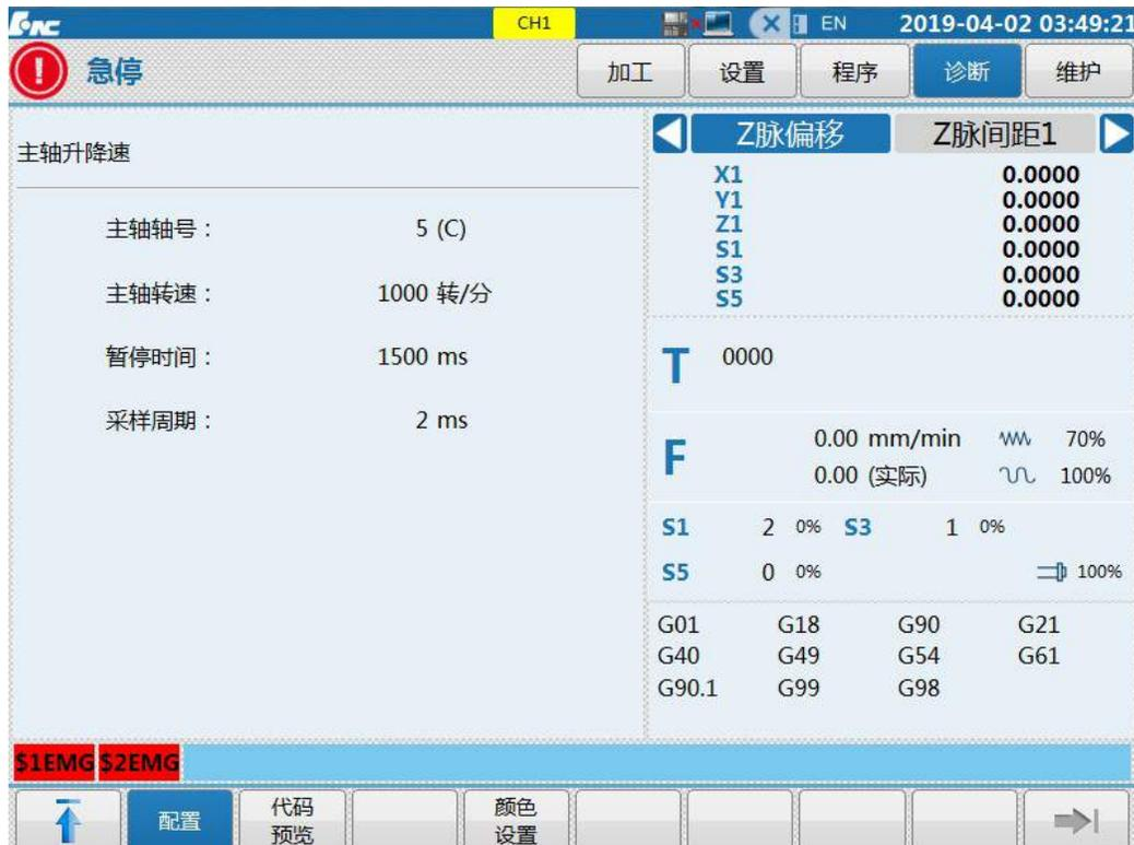
Spindle number: Logical axis number of PWM spindle;
