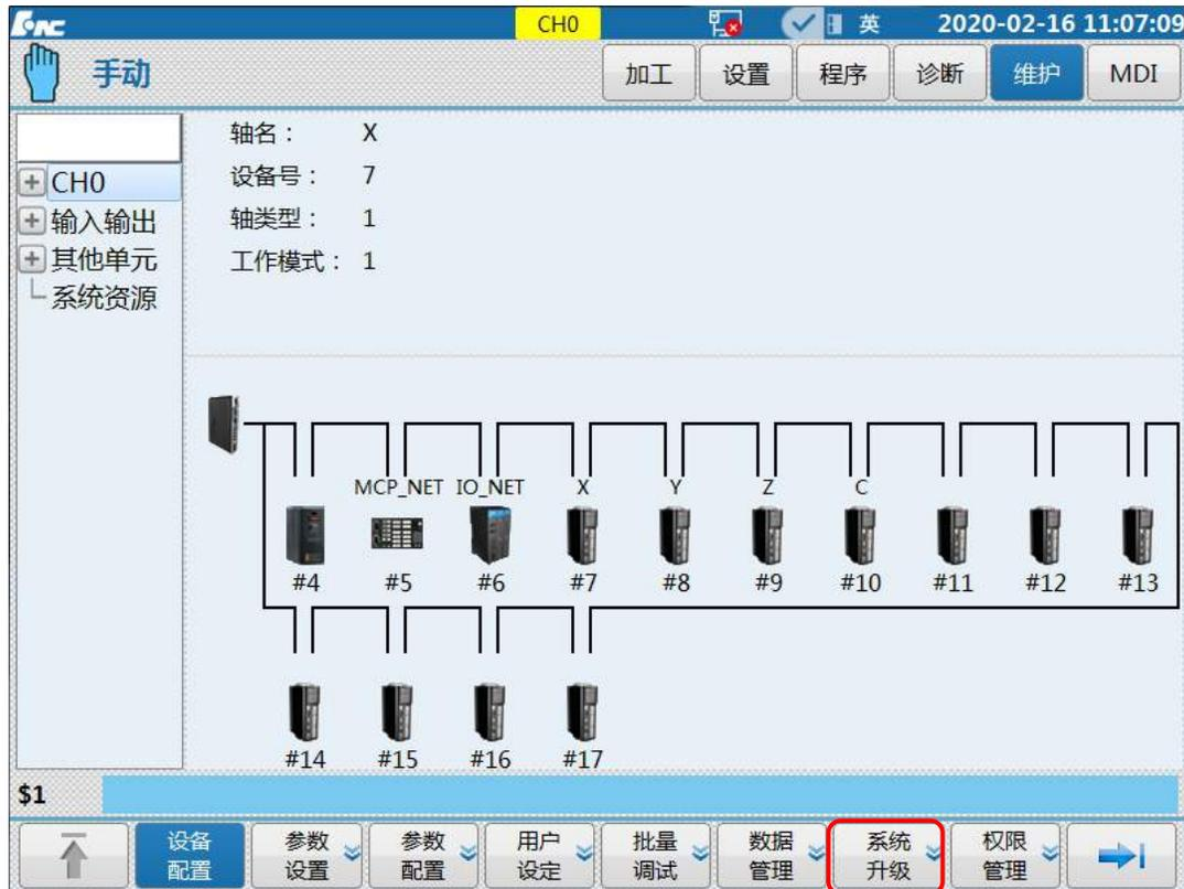
3) Press "Window switch" to switch to upgrade option and select "Type of upgrade option" and "Backup or not" by "↑", "↓", "←" and "→" on the NC panel: Application program, parameter, PLC and BTF. Generally, BTF upgrade is selected and then press "Enter" on the NC panel to confirm. Backup or not: Select based on the actual situation. After selection, "√" is displayed in front of the corresponding option.
