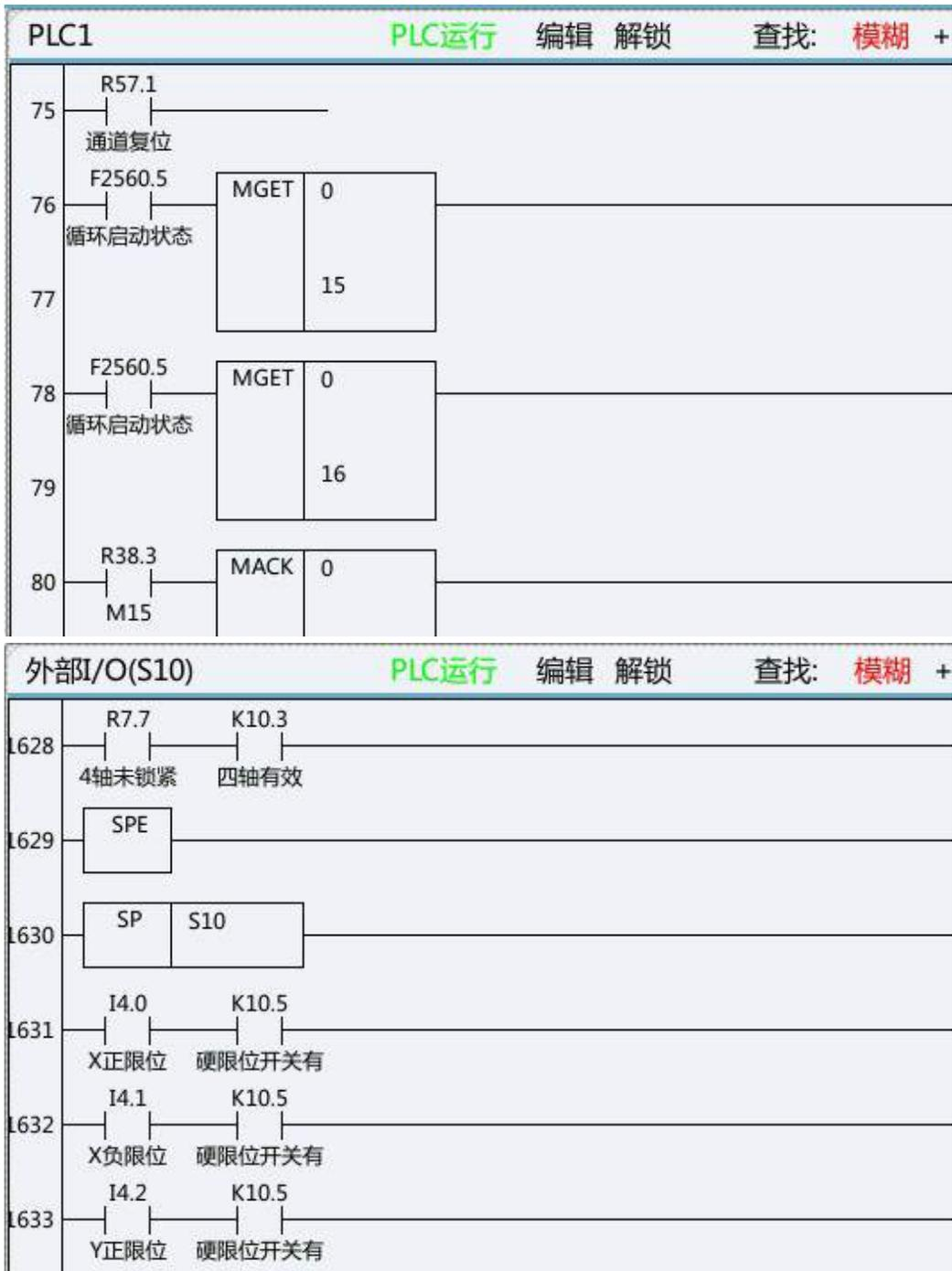
Move the cursor to line 76 or line 1631, press Double coil, and the system will display R0.0 register as double coil output automatically.
