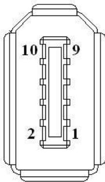
The second position feedback signal input interface socket (facing socket)
