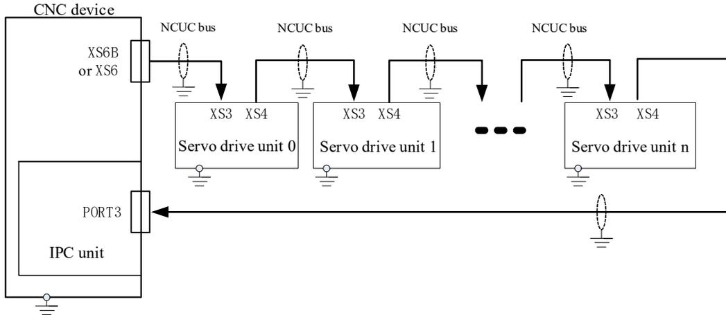
Fig. 2.1 Connection diagram of CNC controller and bus-type servo drive unit
