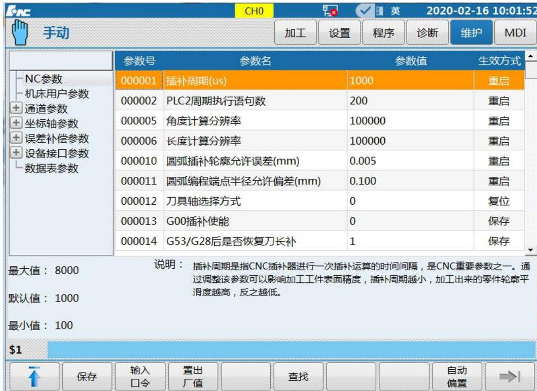
1) PARM000013, "G00 interpolation enable", the parameter is used to determine whether to enable G00 interpolation motion just like G01 interpolation motion.
