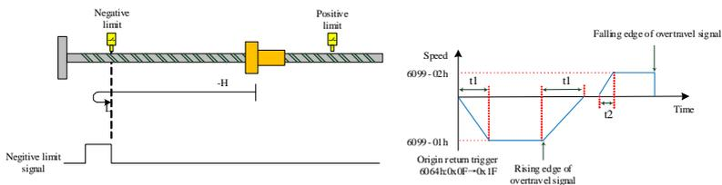
$$t_1 = \frac{6099 - 01h}{609Ah} (s), t_2 = \frac{6099 - 02h}{609Ah} (s)$$
