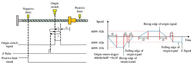
$$t_1 = \frac{6099 - 01h}{609Ah} (s), t_2 = \frac{(6099 - 01h) - (6099 - 02h)}{609Ah} (s), t_3 = \frac{6099 - 02h}{609Ah} (s)$$
