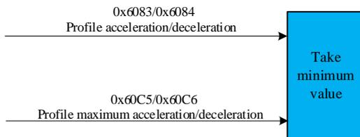
Example: If a 23-bit motor is used and the gear ratio is set to 1:1, if the motor is required to move 10 turns, then the motor speed is 600 rpm, the user acceleration is 600 rpm/s, and the user deceleration is 300 rpm/s.
