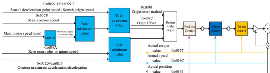
The conversion of user unit and encoder unit in home return mode via 0x6091 is illustrated as follows:
