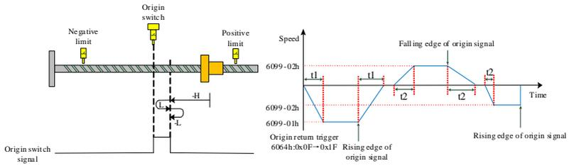
$$t_1 = \frac{6099 - 01h}{609Ah} (s), t_2 = \frac{6099 - 02h}{609Ah} (s)$$
