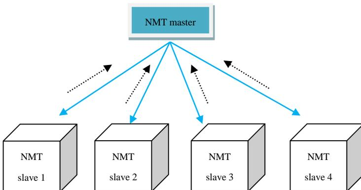
The NMT master sends the remote frame of node protection every 100Ch, and the slave must response, otherwise the slave is considered to be disconnected; if the slave does not receive the node protection remote frame within 100Ch × 100Dh, the master is considered to be disconnected. The NMT master sends remote frames in the format shown in Table 11-12.
