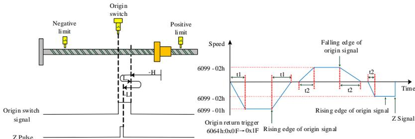
$$t_1 = \frac{6099 - 01h}{609Ah} (s), t_2 = \frac{6099 - 02h}{609Ah} (s)$$
