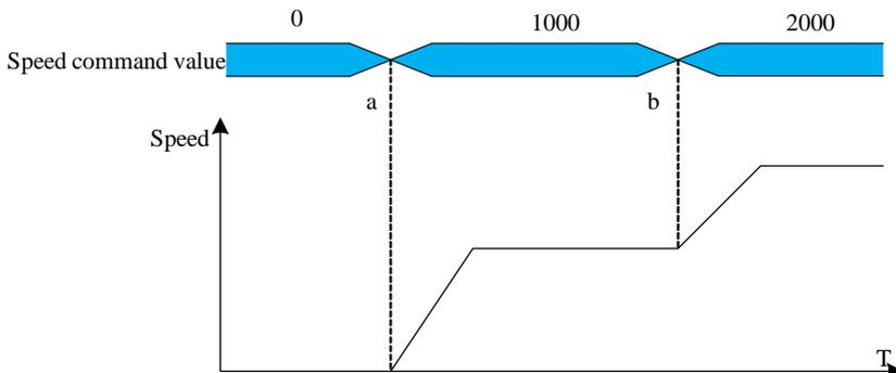
The timing diagram shown in Figure 11.21 corresponds to the operation steps shown below:
