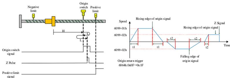
$$t_1 = \frac{6099 - 01h}{609Ah} (s), t_2 = \frac{6099 - 02h}{609Ah} (s)$$
