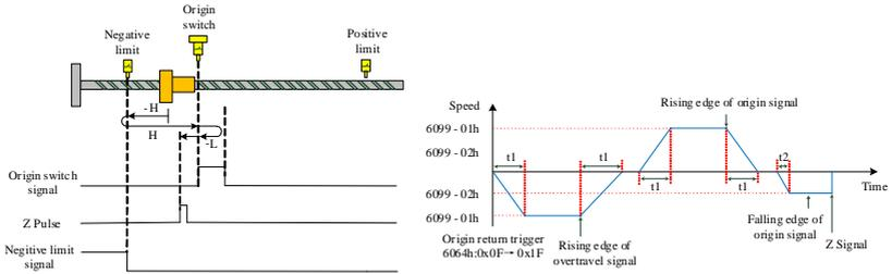
$$t_1 = \frac{6099 - 01h}{609Ah} (s), t_2 = \frac{6099 - 02h}{609Ah} (s)$$
