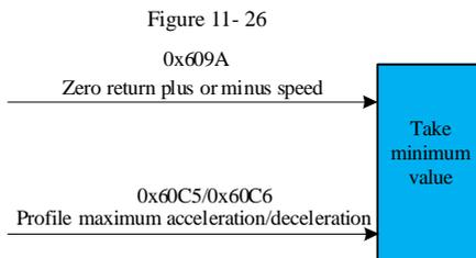
Example: gear ratio = 1:1 with 23-bit encoder. Motor deceleration = 500rpm/s (corresponding to 0x609A (load axis deceleration)) =  $500 * 8388608 / 60 = 69905066$  (command unit/s<sup>2</sup>).
