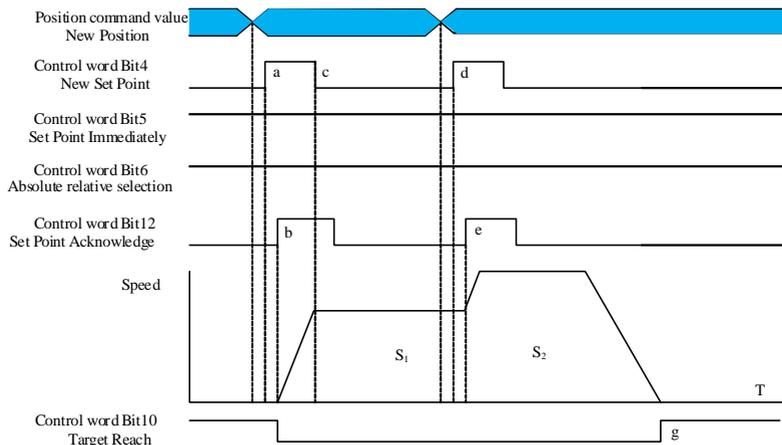
0x6040: bit5=1 immediate change mode ,run the 1<sup>st</sup> stage S1 position command, and before its completion, 0x6040: bit4 and then bit12 are changed into 0 from 1, this means new position command S2 needs to be changed. When 0x6040:bit4 and then bit 12 are changed into 1 from 0, that means new position command is changed and will be performed immediately.
