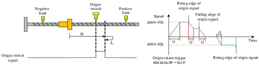
$$t_1 = \frac{6099 - 01h}{609Ah} (s), t_2 = \frac{(6099 - 01h) - (6099 - 02h)}{609Ah} (s), t_3 = \frac{6099 - 02h}{609Ah} (s)$$
