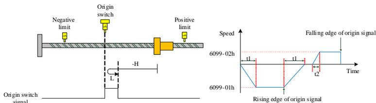
$$t_1 = \frac{6099 - 01h}{609Ah} (s), t_2 = \frac{6099 - 02h}{609Ah} (s)$$
