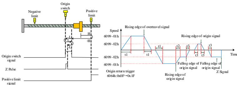
$$t_1 = \frac{6099 - 01h}{609Ah} (s), t_2 = \frac{(6099 - 01h) - (6099 - 02h)}{609Ah} (s), t_3 = \frac{6099 - 02h}{609Ah} (s)$$
