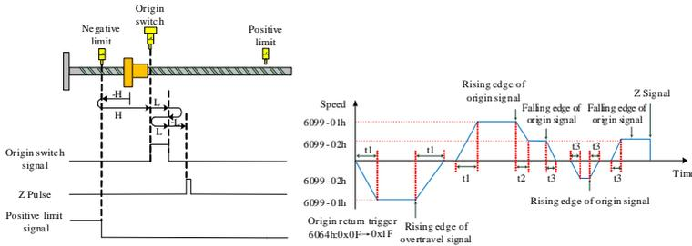
$$t_1 = \frac{6099 - 01h}{609Ah} (s), t_2 = \frac{(6099 - 01h) - (6099 - 02h)}{609Ah} (s), t_3 = \frac{6099 - 02h}{609Ah} (s)$$
