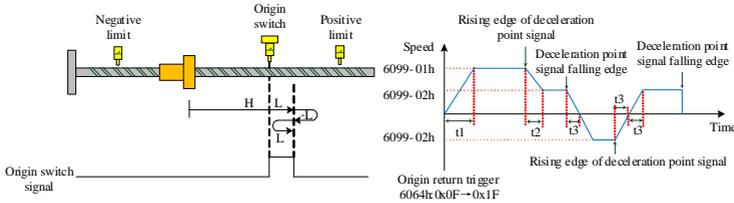
$$t_1 = \frac{6099 - 01h}{609Ah} (s), t_2 = \frac{(6099 - 01h) - (6099 - 02h)}{609Ah} (s), t_3 = \frac{6099 - 02h}{609Ah} (s)$$
