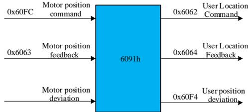
$0x6091(\text{gear ratio}) = \frac{\text{motor resolution}}{\text{load resolution}} \cdot 0x6063(\text{motor position feedback})$  and  $0x6064(\text{user location feedback})$  relationship is :  $0x6063(\text{encoder unit}) = 0x6064(\text{command unit}) \times \text{gear ratio}$ .
