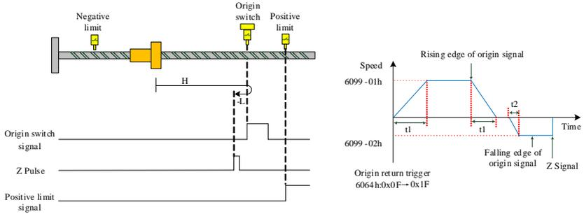
$$t_1 = \frac{6099 - 01h}{609Ah} (s), t_2 = \frac{6099 - 02h}{609Ah} (s)$$
