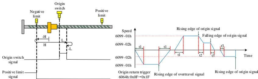
$$t_1 = \frac{6099 - 01h}{609Ah} (s), t_2 = \frac{(6099 - 01h) - (6099 - 02h)}{609Ah} (s), t_3 = \frac{6099 - 02h}{609Ah} (s)$$
