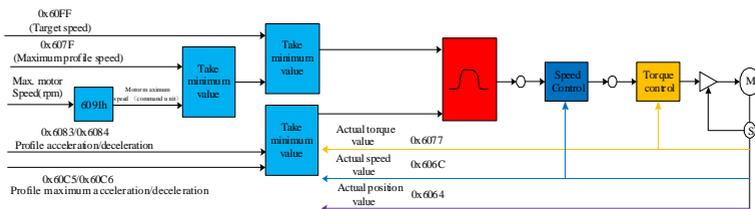
The conversion of user units and encoder units in profile velocity mode via 0x6091 is illustrated below:
