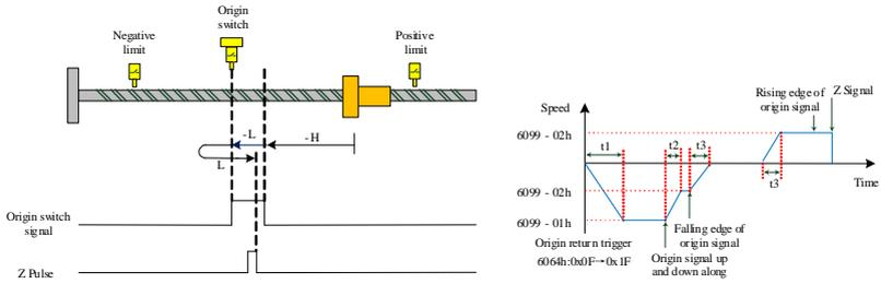
$$t_1 = \frac{6099 - 01h}{609Ah} (s), t_2 = \frac{(6099 - 01h) - (6099 - 02h)}{609Ah} (s), t_3 = \frac{6099 - 02h}{609Ah} (s)$$
