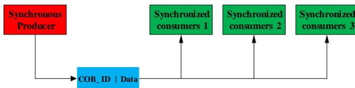
The synchronization in Canopen is realized by sending control data to each slave with PDO. Each slave that receives control commands from the master only saves the commands temporarily, and only after all the slave commands are sent will the master send out a synchronization (SYNC) broadcast message, and all slaves that support synchronization transmission mode will execute the previously received control commands at the same time after they have received the synchronization (SYNC) message.
