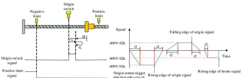
$$t_1 = \frac{6099 - 01h}{609Ah} (s), t_2 = \frac{6099 - 02h}{609Ah} (s)$$
