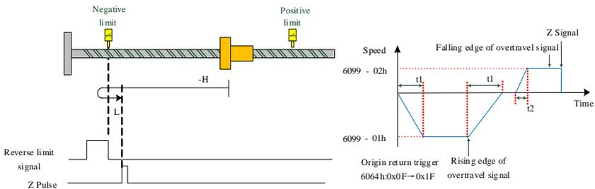
$$t_1 = \frac{6099 - 01h}{609Ah} (s), \quad t_2 = \frac{6099 - 02h}{609Ah} (s)$$
