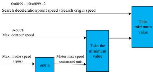
Motor speed (rpm) versus load shaft speed (command unit/s):
