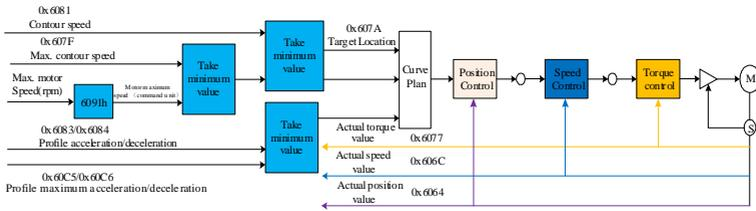
The conversion of user and encoder unit in profile position mode via 0x6091 is illustrated as follows:
