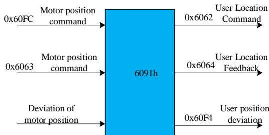
$$0x6091(\text{gear ratio}) = \frac{\text{motor resolution}}{\text{load resolution}}$$
