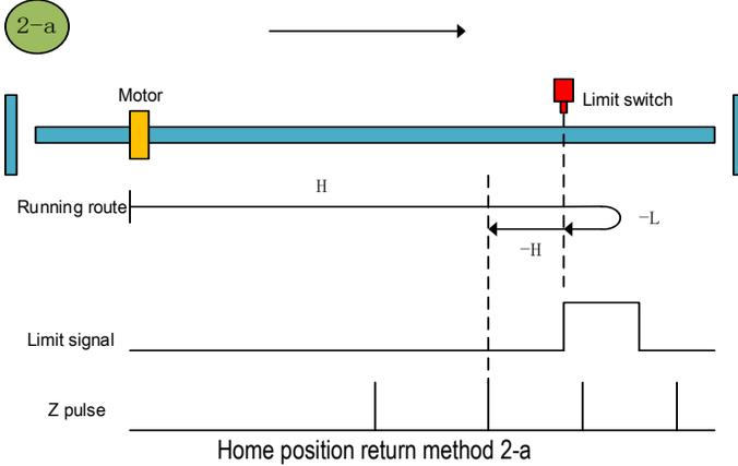
b. Start the home position return → forward limit valid → search for the falling edge of forward limit at low speed reverse direction → search for Z pulse in reverse direction.
