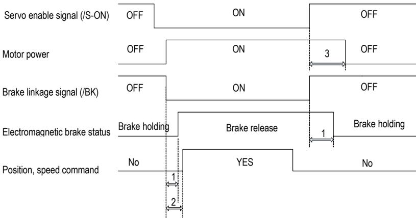
1. Different types of brakes may have slight difference on the time of holding brakes and loosening brakes.
