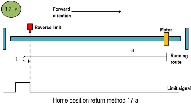
b. Start the home position return → Reverse limit valid → Stop after searching for the falling edge of reverse limit at low speed forward direction.
