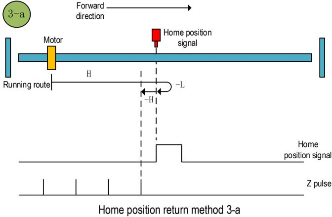
b. Start the home position return → Home position signal ON → Search for the falling edge of home position signal at low speed reverse direction → search for Z pulse in reverse direction.
