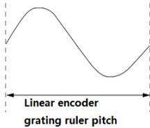
The grating ruler pitch of linear encoder = 1 cycle distance of analog voltage feedback signal sent by linear encoder.
