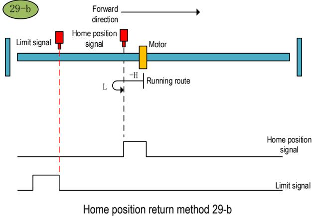
c. Start the home position return → Home position signal OFF → Search for the falling edge of home position at high speed reverse direction → Touch the reverse limit → Search for the rising edge of home position at high speed forward direction → Decelerate to 0 → Search for the falling edge of home position at low speed reverse direction → Stop after searching for the rising edge of home position at low speed forward direction.
