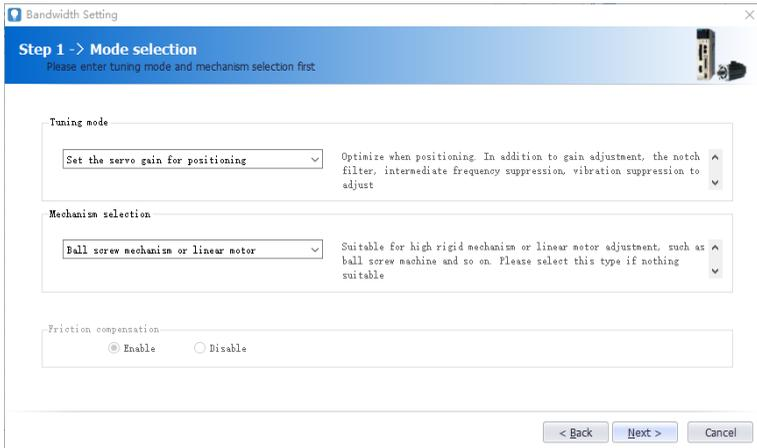
b). Click on [Next] to enter the setting interface of inertia moment ratio and set the inertia ratio (inertia ratio can be obtained through inertia identification function).
