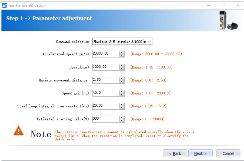
b). As shown in the above figure, set the corresponding parameters according to the actual situation (usually keep the default), and click [Next] → [Write] → [Next] → [Enable] → [Forward] → [Reverse] After the forward rotation is repeated three times, the final inertia identification result is displayed, as shown in the following figure.
