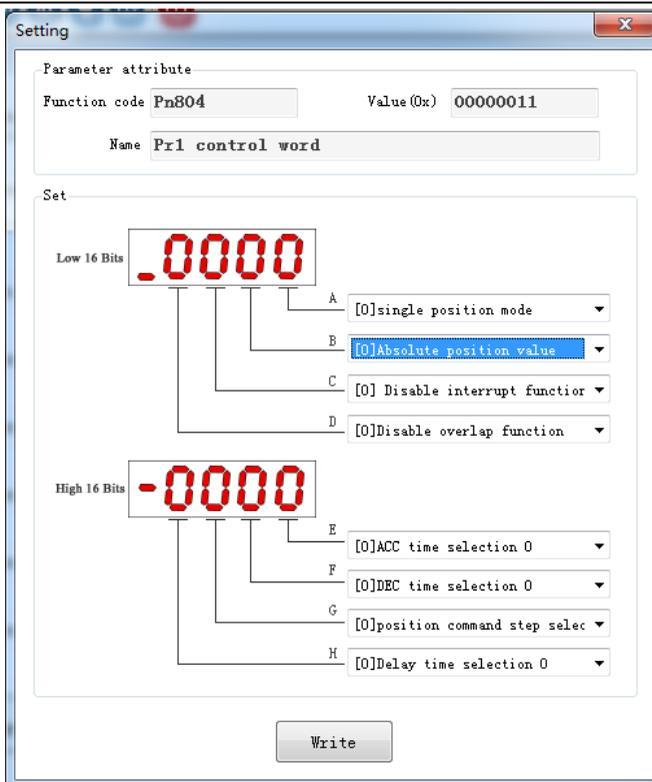
Function code A part function definition: select internal position mode.
