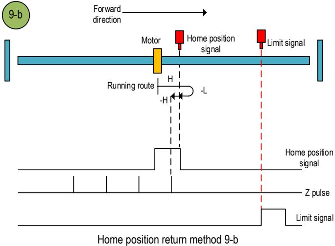
c. Start the home position return → Home position OFF → Search for the falling edge of home position at high speed forward direction → Touch the forward limit → Search for the rising edge of home position at high speed reverse direction → Decelerate to 0 → Search for the falling edge of home position at low speed forward direction → Search for the rising edge of home position at low speed reverse direction → Search for the Z pulse in reverse direction.
