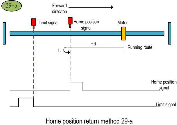
b. Start the home position return → Home position signal ON → Search for the falling edge of home position at high speed reverse direction → Decelerate to 0 → Stop after searching for the rising edge of home position at low speed forward direction.
