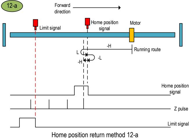
b. Start the home position return → Home position signal ON → Search for the falling edge of home position at low speed forward direction → Search for the rising edge of home position at low speed reverse direction → Search for the Z pulse in reverse direction.
