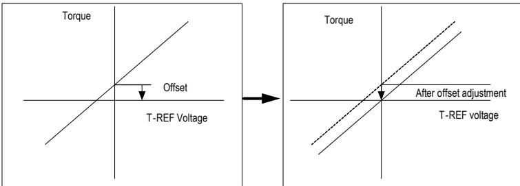
There are two methods of automatic adjustment and manual adjustment of offset adjustment. Automatic adjustment is automatically adjusting the command offset (Fn100) and manual adjustment is manually adjusting using command offset (Fn102). For details, see "Auxiliary Functions".
