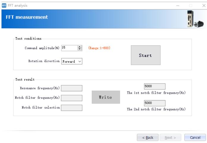
b). Click on [Start] to measure the first notch, and then click on [Write] to write the frequency of the first notch filter.
