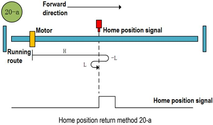
b. Start the home position return → Home position signal ON → Search for the falling edge of home position at low speed reverse direction → Stop after searching for the rising edge of home position at low speed forward direction.
