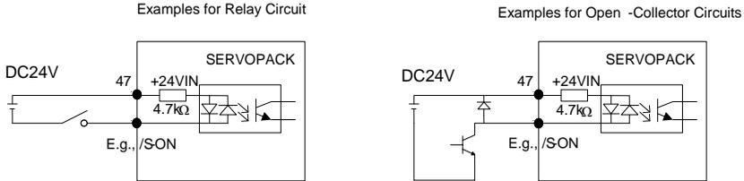
**Note:** The external power supply (DC24V) must have a capacity of 50 mA or more. The input loop of the servo unit uses a bidirectional optocoupler. Please select the sink circuit connection or the source circuit connection according to the specifications of the machine.
