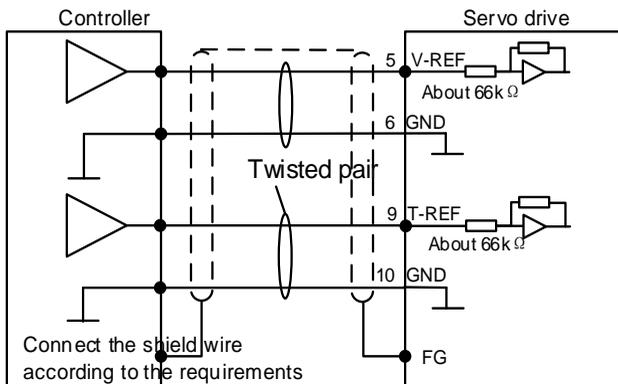
The above wiring is an example of wiring during forward rotation.
