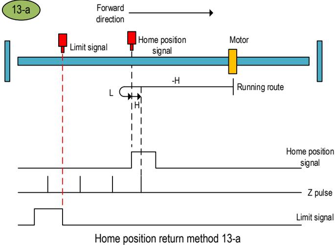
b. Start the home position return → Home position signal ON → Search for the falling edge of home position at high speed reverse direction → Decelerate to 0 → Search for the rising edge of home position at low speed forward direction → Search for the Z pulse in forward direction.
