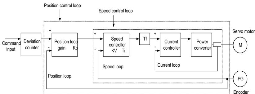
Please adjust each servo gain one by one after fully understanding the composition and characteristics of the servo units if the servo gain needs to be adjusted manually. In most cases, if one parameter changes significantly, the other parameters must be adjusted again. In order to confirm the response characteristics, preparations must be made to observe the output waveform of the analog monitor using a measuring instrument.
