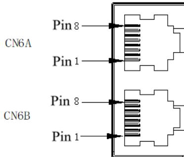
According to different models, the definition of the port is different. When using it, you need to confirm the model before defining the interface. For model identification, please refer to “1.6 driver naming”. The field identification bit E is P: pulse type; S: standard type; C: CANopen bus type; N: PROFINET bus type.
