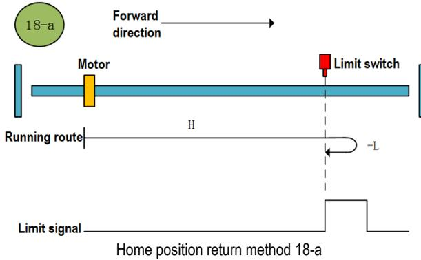
b. Start the home position return → Forward limit valid → Stop after searching for the falling edge of forward limit at low speed reverse direction.
