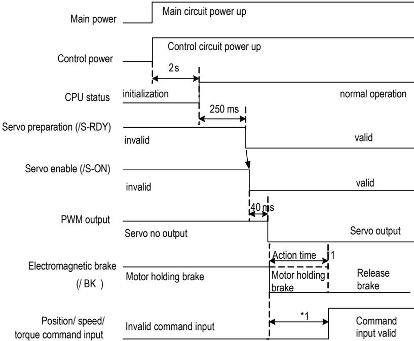
1: There is a delay in the electromagnetic brake operation. The operation time varies depending on the type of brake. It is recommended to be more than 100ms to ensure that the electromagnetic brake is completely released when the command is input. This time can be omitted when motor is not braked.
