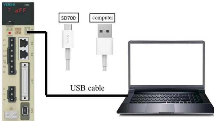
1. Connection between PC and SD700 servo drive via Android micro mobile phone data cable.
