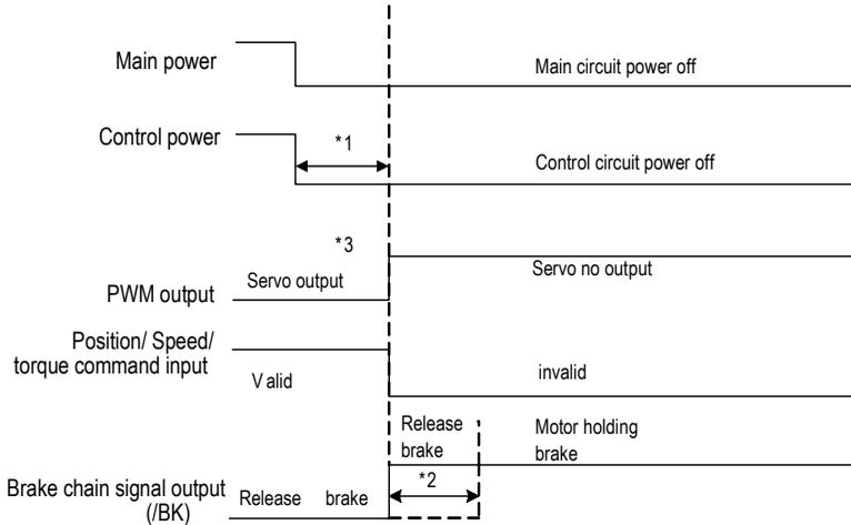
1. Undervoltage fault occurs when the control power supply voltage drops below 170V/350V (220V series, 400V series).
