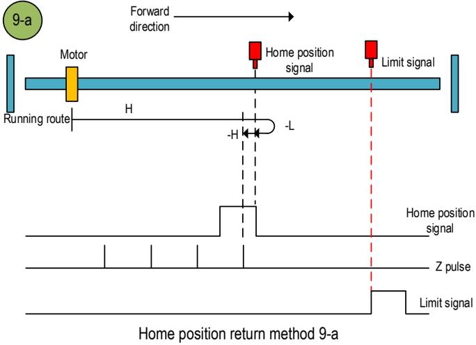
b. Start the home position return → Home position signal ON → Search for the falling edge of home position at high speed forward direction → Decelerate to 0 → Search for the rising edge of home position at low speed reverse direction → Search for the Z pulse in reverse direction.
