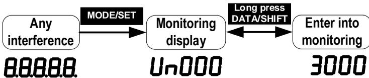
If you want the monitor to automatically display related information after the servo drive is powered on, set PN003 (default 0xFFF) to a relevant value. For example, if you want the motor speed to automatically display after the drive is powered on, set PN003 to 00000 (motor speed). For details about the values of each monitoring information, see "Monitor Display".
