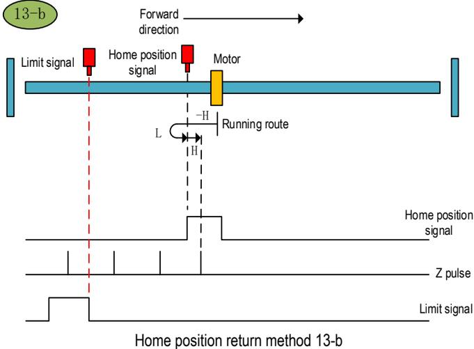
c. Start the home position return → Home position signal OFF → Search for the falling edge of home position at high speed reverse direction → Touch the reverse limit → Search for the rising edge of home position at high speed forward direction → Decelerate to 0 → Search for the falling edge of home position at low speed reverse direction → Search for the rising edge of home position at low speed forward direction → Search for the Z pulse in forward direction.
