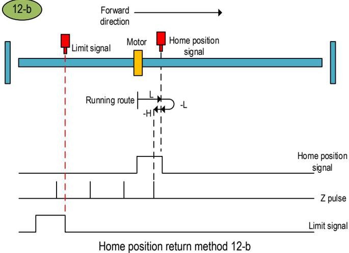
c. Start the home position return → Home position signal OFF → Search for the rising edge of home position at high speed reverse direction → Touch the reverse limit → Search for the falling edge of home position at high speed forward direction → Decelerate to 0 → Search for the rising edge of home position at low speed reverse direction → Search for the Z pulse in reverse direction.
