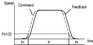
When the switching condition of the mode switch is set as acceleration, if the speed command exceeds the acceleration set in Pn134, the speed loop will be switched to P control.
