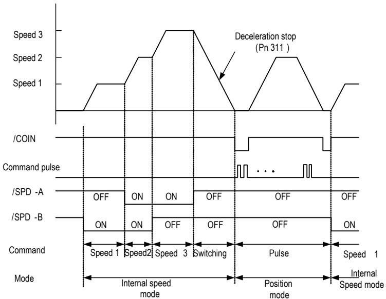
Note : The internal speed mode is decelerated during the deceleration time set by Pn311 to stop the motor, then switch to the position mode
