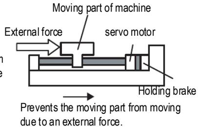
The brake has the following operation delay time. ON and OFF of the operation, please ensure the brake operation time.
