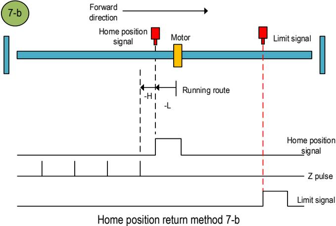
c. Start the home position return → Home position OFF → Search for the rising edge of home position at high speed forward direction → Touch the forward limit → Search for the falling edge of home position at high speed reverse direction → Decelerate to 0 → Search for the rising edge of home position at low speed forward direction → Search for the falling edge of home position at low speed reverse direction → Search for the Z pulse in reverse direction.
