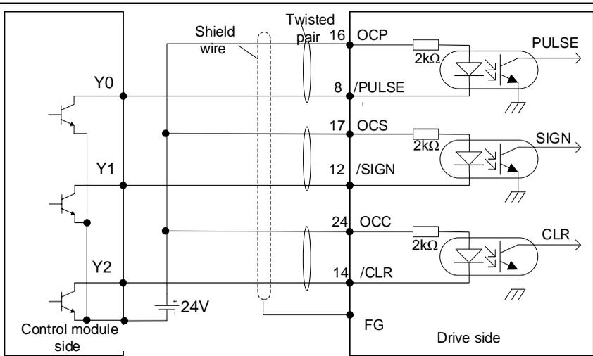
2. Control modules is PNP type (common anode):
