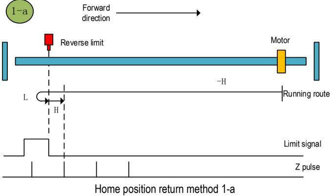
b. Start the home position return → reverse limit valid → Search for the falling edge of reverse limit at low speed forward direction → search for Z pulse in forward direction.
