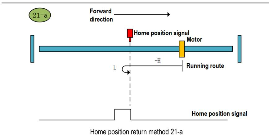
b. Start the home position return → Home position signal ON → Stop after searching for the falling edge of home position at low speed forward direction.
