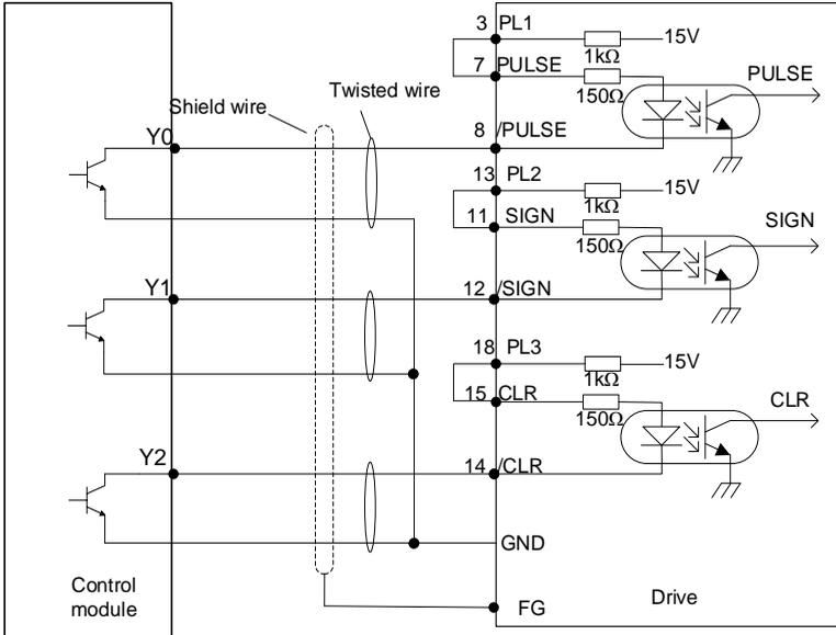
2 Control modules is PNP type (common anode):
