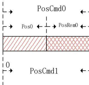
As shown in the figure above, the first position command setting value is PosCmd0. After the pulse of Pos0 is run, the operation ends and the remaining PosRem0 pulses are not completed. If the second absolute position command PosCmd1 is inserted at this time, the total number of pulses of the second position command operation is PosCmd1- Pos0. That is, the second absolute position value PosCmd1 is the absolute position 0 bit reference point, and the final running position value is PosCmd1.
