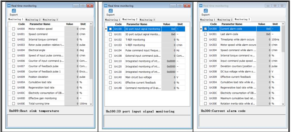
b). Check the monitored parameters and monitor the servo. During the monitoring process, you can also export and save the monitoring content.
