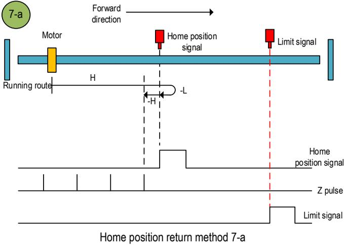
b. Start the home position return → Home position signal ON → Search for the falling edge of home position at low speed reverse direction → Search for the Z pulse in reverse direction.
