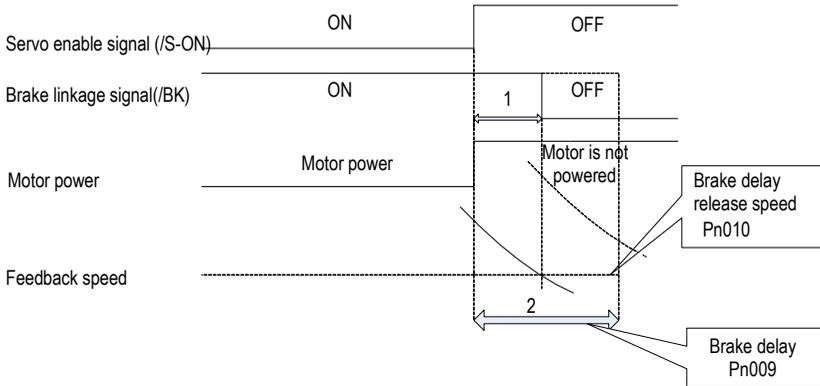
1. When the motor speed is lower than the set value of Pn010 after the power to the servo motor is turned OFF, the /BK signal output time is subject to 1.
