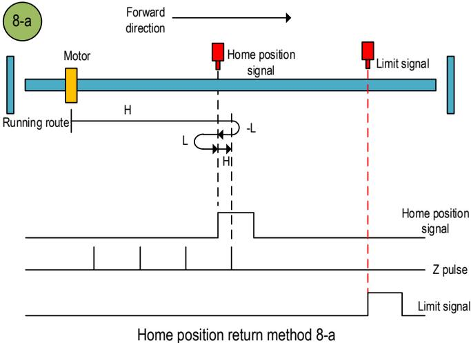
b. Start the home position return → Home position signal ON → Search for the falling edge of home position at low speed reverse direction → Search for the rising edge of home position at low speed forward direction → Search for the Z pulse in forward direction.
