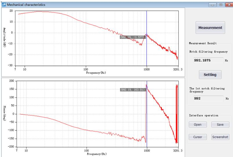
c). From the above figure, you can analyze the frequency, amplitude, and phase of the resonance frequency. Click on [Settings] to set the frequency of the first notch filter. After the setting is completed, the screen is closed. Mechanical properties are completed.
