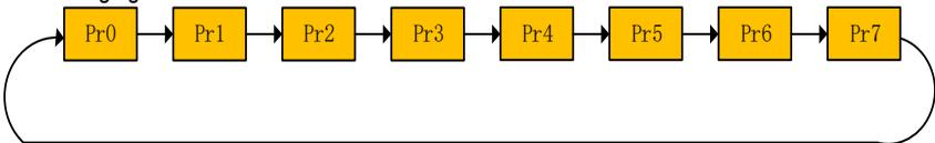
As shown in the figure above, when the Pr command of the last paragraph of the multi-segment position command is set as a jump command, from the last Pr command to the Pr command at the beginning, so that multiple Pr commands can be executed in a loop.
