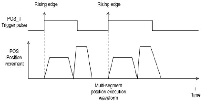
Speed mode description: If the current position command segment is given the speed mode, when the position command is planned, the motor runs at the set speed until the next Pr position command starts.
