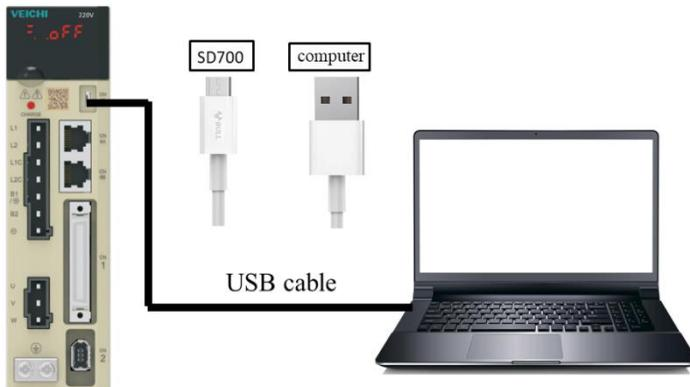
1. Connection between PC and SD780 servo drive via Android micro mobile phone data cable.
