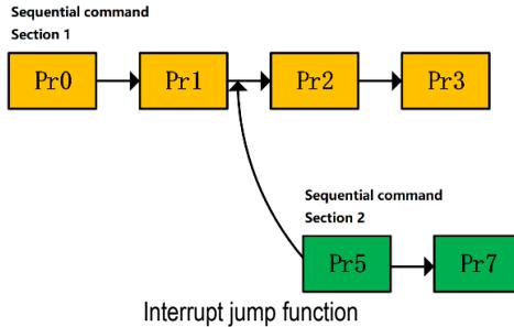
As shown in the figure above, there are two command segments 1 and 2 that are executed sequentially. When multiple segments of command 1 are currently being executed, by external trigger segment 5, and segment 5 is specified by Pr as a jump command, interrupt function is enabled, and jump the target command segment number is 7. The currently running multi-segment command ends and immediately starts to execute the position command value of Pr command segment 7.
